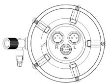
This mode is similar to other ribbon microphones, when you decide to use your favourite mic preamps. In this case you don't need to connect PSU and Remote Controller at all, and have mic level signals directly from RS-2 mic body to your external preamps.
