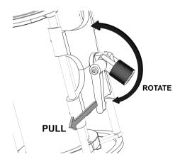
Thanks to the spring mechanism you can tighten or loose the lever fully even when only small rotation angle is possible. To make full use of this feature - just pull the lever towards the grey arrow , rotate to a new required starting position (black arrow ) and release. Then you can continue to tighten or loose the lever.
