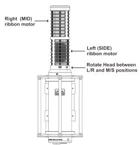
Besides stereo and M/S applications of course you can always use any of the two RS-2 channels for recording mono sources, like vocals. When you decide to record mono source, it is good idea to rotate head to M/S position and turn Remote Controller SIDE gain pot to zero, than sing or play instrument to the upper ribbon. Of course you can be creative here and instead of recording mono track, you can make use of M/S mode and gradually increasing SIDE gain expand the stereo image.
