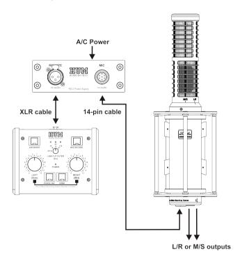
RS-2 microphone set has XLR cable for connecting Remote Controller and special high quality 14-pin cable for connecting PSU included in the RS-2 set. 6 meters of 14-pin cable length should be more than enough in all typical studio situations. In case when you need this cable longer than standard - you can order a
