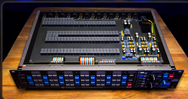
Independent PCB boards for left and right channels...
